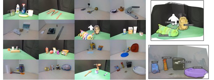
Fig. 6: Sample sequences from the UnCoCo dataset we captured to evaluate long-tailed reasoning over open-set multimodal 3D maps. To the right, we show sample reconstructions and semantic annotations over two sub-sequences. For each scene, UnCoCo provides 2D and 3D segmentation masks, and text, image, click, and audio queries.
