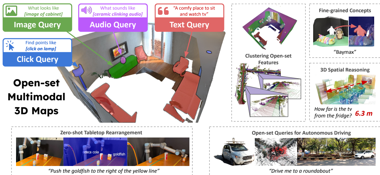
Fig. 1: ConceptFusion presents an approach to build open-set multimodal 3D maps from RGB images and depth estimates from additional sources such as depth/stereo cameras or lidar, and features from foundation models like CLIP, DINO, AudioCLIP, etc. These maps are built online, and can be queried for arbitrary concepts specified as text, images, audio samples, or clicks on the 3D map. The fused features have an implicit understanding of semantic concepts, as evident by visualizing clusters obtained from a K-means algorithm. ConceptFusion features are significantly more adept at retaining fine-grained concepts, such as the disney character “Baymax”. We also build 3D spatial reasoning modules that enable reasoning about frequently observed spatial relationships. We demonstrate the applicability of ConceptFusion to the real-world robotic tasks of tabletop manipulation of novel objects, and an urban autonomous driving setting. (Webpage)
